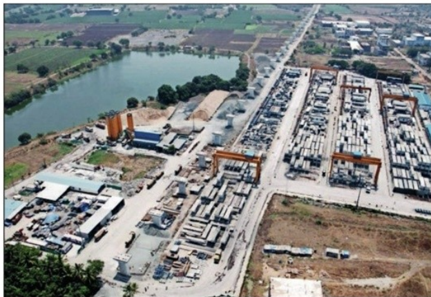
Nearly 92% of the bullet train corridor will be elevated. So NHSRCL has set up a segmental casting yard at Surat to make spans
